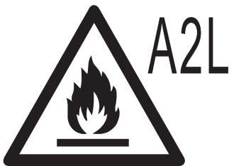
Caution:Risk of fire
