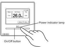
The Power indicator lamp remains lit while the indoor unit is operating.
