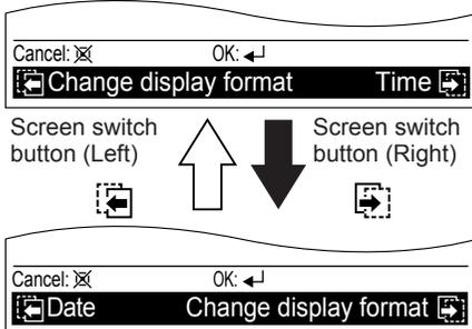
**NOTE:** These buttons are active only when any combinations of or and the relevant screen names are displayed in the black field at the bottom of the screen.
