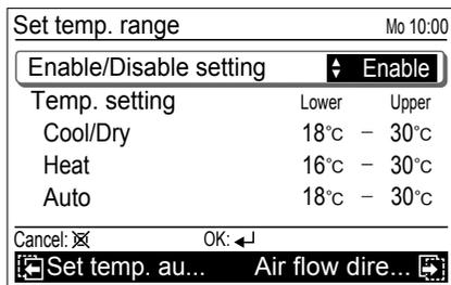
**4** For [Temp. setting], select mode with the [Cursor button (Up/Down)] and press the [Enter button]. Adjust [Lower] and [Upper] value with the [Cursor button (Up/Down)]. With the [Cursor button (Left/Right)], the cursor can be switched [Lower] and [Upper]. To complete the setting, press the [Enter button].
