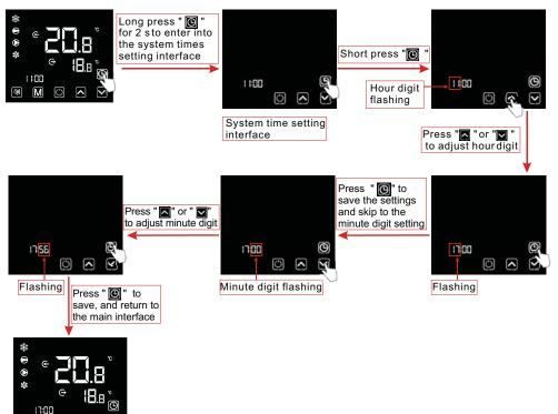
Notes: Under the clock setting interface, if there is no operation for 20 s, the system will automatically memorize use' s settings, and return to the main interface; if short press is during any operating steps, the changes will not be saved and return to the main interface.
