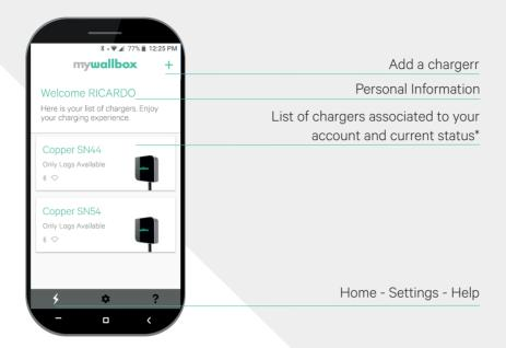
\*Enter the Serial Number (SN) and the Unique Identifier (UID) you'll find on the lable located on the bottom of the charger. When connection is done, you'll be able to manage your charger.
