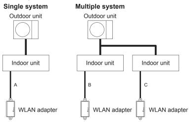
A, B, and C: Shielded cable attached to this product.
