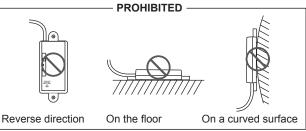
Do not lay the WLAN adapter cable on the floor. You may trip on the cables.
