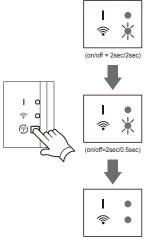
**7** Press [Register] to start the connection with the wireless router.
