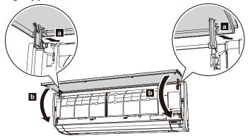
(4) Press 4 places on the intake grille to close it completely.
