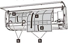
(3) Filter holder and air cleaning filter are attached on the rear side of the air filter. Remove them from the air filter by unlatching each corner of the filter holder [d].
