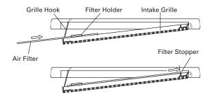
5. Close the intake grille and push the intake grille's hooks outward.
