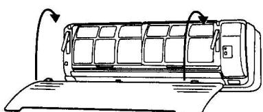
2. Press the both lower sides of the intake grille until you hear a clicking sound and the grille locks into place.
