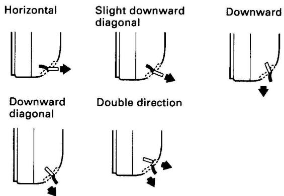
In order to heighten the efficiency of cooling and drying modes, the airflow-direction louvers should be set within the following ranges:
