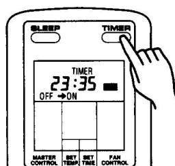
**3 Press the TIMER button to select the PROGRAM Timer operation ( OFF → ON or OFF ← ON will display).**
