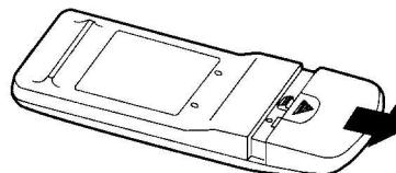
Slide in the direction of the arrow while pressing the  mark.
