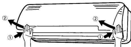
Press the both lower sides of the intake grille until you hear a clicking sound and the grille locks into place.
