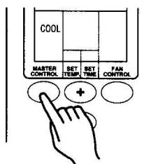
If you wish to change operating conditions (Mode, Fan Speed, Thermostat Setting, Air flow direction), after making the timer setting wait until the entire display reappears, then press the appropriate buttons to change the operating condition desired.
