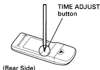
Use the tip of a ball-point pen or other small object to press the button.
