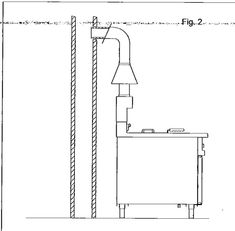
To connect the appliances to a flue that expels the waste gas into the outside atmosphere, see the illustration.
