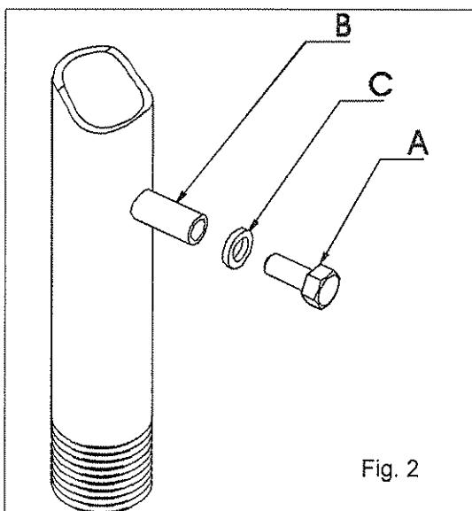
Gas supply pressure must be measured at the pressure point (Ref. B) after removing the sealing screw (Ref. A). Use a flexible pipe, connect a gauge e.g. a liquid gauge that is accurate to 0.1 mbar) to the pressure point (and measure the intake pressure whilst the appliance is operating. If the pressure reading does not fall within the upper and lower limits indicated on the table, the appliance cannot be installed.
