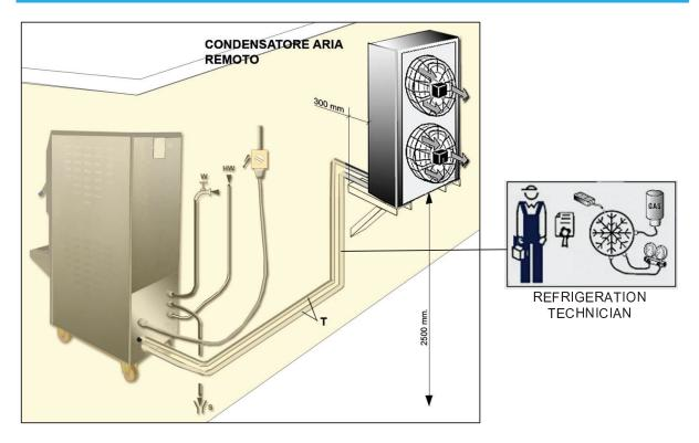
To avoid air overheating problems, when possible, mount the remote air condenser.
