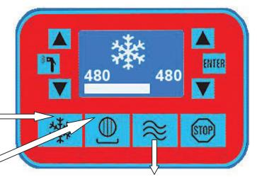
If we want to remove the ice-cream at low speed and without cooling, press this key.
