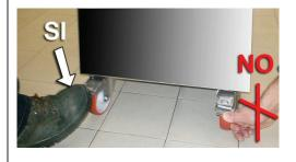
Move the machine by holding the handle of the flange with one hand and the corner of the machine with the other hand.
