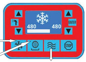
If wanting to remove the ice-cream at low speed and without cooling, press this key.
