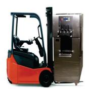
Hoist the machine using a fork lift truck, inserting the forks from the side of the machine between the front and rear wheels.
