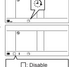
(2) Set enabled with the [+] or [-] buttons. Then press the [→ ENTER] button. If set to "Enable", proceed to (3). If set to "Disable", return to "Monitor Mode Screen".
