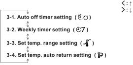
Returns to this screen after setting. Return to "Monitor Mode Screen" if the [■ MENU] button and [ < ] button pressed and held simultaneously for at least 2 seconds.
