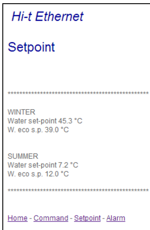
Figura 35. Pantalla “Set point” ethernet.
