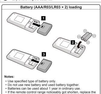
batteries, and press RESET button.
