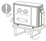
If it is damaged, it may lead to the fall of the unit and cause the injury.
