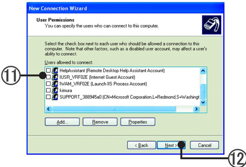
⑪ This screen sets the users who can connect to the computer. The users of the Operating System of the machines set at “Users allowed to connect” are displayed. Check the users allowed to connect from the displayed list. (\*1) Verification is performed by the Operating System at incoming. For connection from the client, the user set here and the password of that user must be inputted. (\*2) Information
