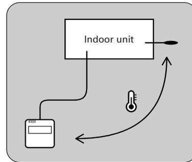
Press the ECONOMY button for more than 2 seconds to select whether the room temperature is detected at the indoor unit (remote sensor) or the remote controller.
