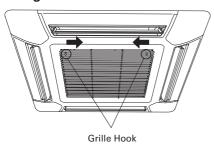
2. Pull out the filter from the intake grille.
