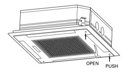
Hold down the hook at A and pull the filter out.
