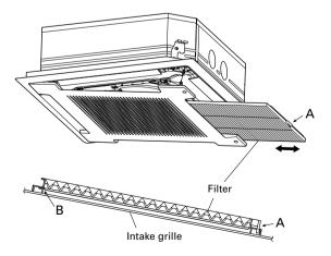
When reinstalling the filter, be sure that the hooks at A and B engage correctly into place.
