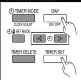
Press the DAY (DAY OFF) button and SET button simultaneously for 2 seconds or more to activate the child lock function and lock all buttons on the remote controller. Press the buttons again for 2 seconds or more to deactivate the child lock function.
