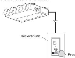
Press the MANUAL AUTO ( 1/0 ) button on the receiver unit control panel.
