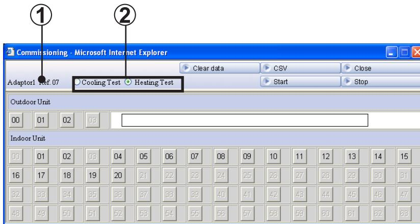
③ Select the unit which is to start test run. Select the unit by clicking the button of the relevant unit No.
