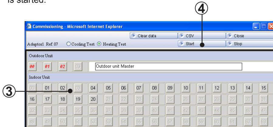
⑤ The button of units that have entered the test run state is displayed in green. When an indoor unit was selected and started, the selected indoor units enter the test run state. When an outdoor unit was selected and started, all the indoor units enter the test run state.
