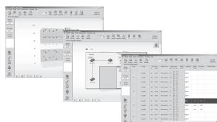
Monitoring of indoor unit operation can be performed using any one of three patterns: 3D display, floor layout display, list display, set temperature and turning the indoor units on and off.
