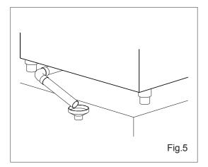
For connection to the drain outlet, install the funnel (supplied with the appliance) in order to ensure that the water drains off freely. The drain tube must always be open in order to avoid problems of pressure in the chamber (Fig. 5).
