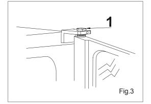
Check that the door closes correctly and that the seal between the door and the oven compartment is correctly positioned. If necessary, adjust the door hinges in order to ensure that the oven is air-tight when in operation.
