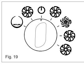
The cooling cycle can be interrupted at any time by turning the programme selector knob to the position shown in fig. 19.
