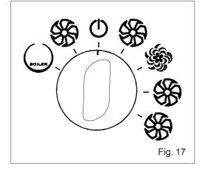
At the end of the cooking cycle, turn the selector knob to the position shown in Fig. 17.
